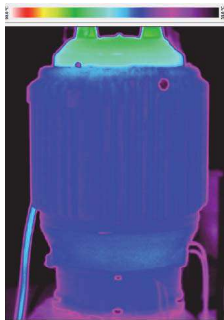
Thermal view of a 55kW motor after 6 hours of continuous operation under full load and at maximum permissible operating temperature
